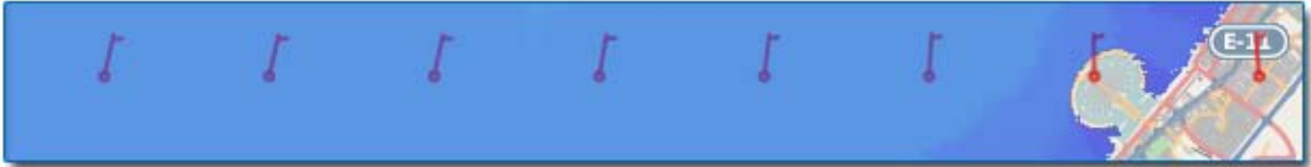
Figure 5-2 Map with winds and wave height layers enabled (barbs point in the direction the wind is coming from)
